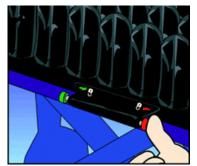
STEP 8 Position user on the cushion in their desired posture and have them maintain this position while air transfers through the ISOFLO Memory Control. Once the air transfer is complete, push the ISOFLO's "Red" knob toward the left, in the LOCKED position. This will isolate the flow of air and provide a more stable sitting position. Recheck each compartment of the cushion to ensure proper inflation.
