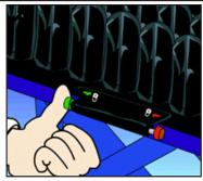
STEP 2 Make sure the ISOFLO Memory Control is also open by pushing ISOFLO's Green Knob to the right or "UNLOCKED".
