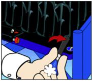
STEP 4 Pinch pump's nozzle and turn valve **clockwise** to close. Remove pump.
